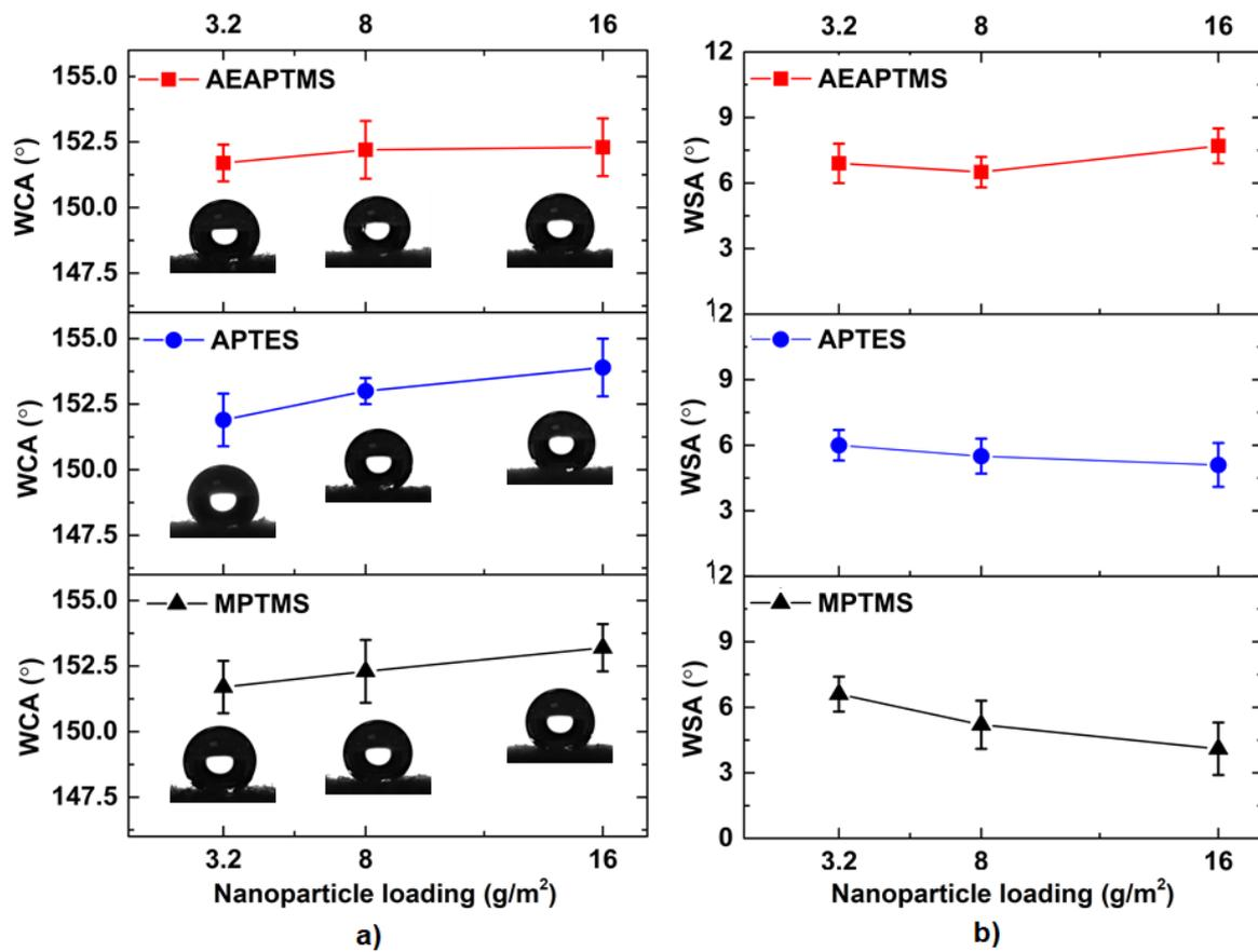
**Fig. 3.** The effect of nanoparticle loading on a) WCA and b) WSA for the as-prepared fabrics treated with AEAPTMS, APTES and MPTMS.
